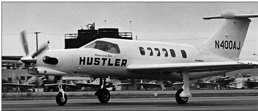
The 1970s Hustler, "a somewhat controversial concept." This airplane was designed for single-pilot operation and was originally planned to have a P&W PT6 turboprop in the nose and a P&W JT15D jet in the tail. The rear-mounted jet was never installed and the Hustler didn't make it into production.
